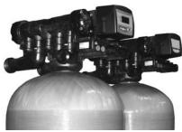
Safe Water Technologies' Commercial Water Softeners are built utilizing SWT's ProSoft™ resin as the primary layer. These cationic ion exchange systems are designed to remove calcium and magnesium (hardness), and a host of other cations from the water. SWT takes care of the little extras such as: machined PVC distribution systems, oversized brine tanks, safety float for 16 inch or larger systems, and an anthracite underbedding for
